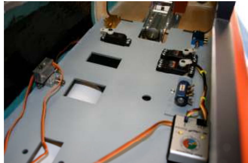
photo 14 – sample layout of air systems on forward component board .. leave room for cockpit above and air tanks below
