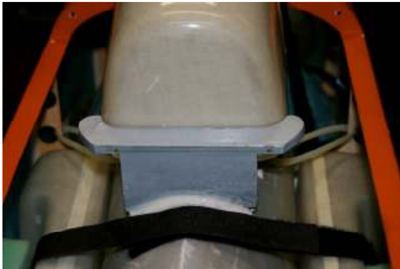
photos 8 and 9 – securing intake and rear tank stop
