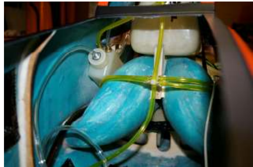
photos 10 and 11 – vent tube reinforcement and UAT installation
