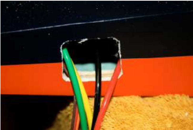
photo 26 – enlarge air line and servo wire access hole in wing root
