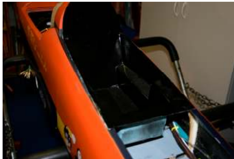
photo 30 – trim the sides of the cockpit area such that the tubs drop in place
