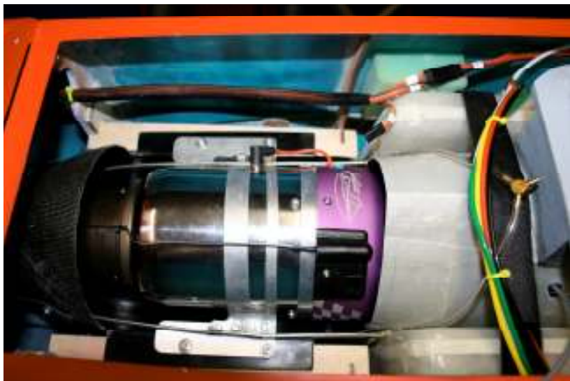
photo 23 – engine mounted in lower bypass
