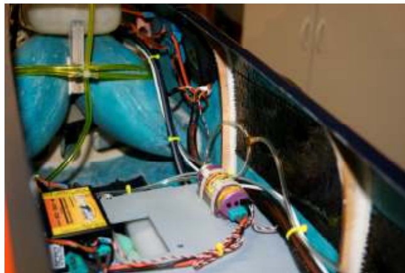
photos 24 and 25 – rear component board. Note receiver position on upper right.
