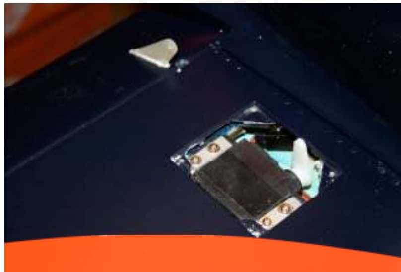
photo 17 – elevator servo installation
