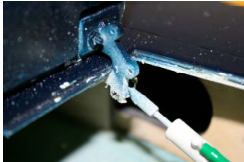
photo 27 – optional repositioning of main door cylinder attach bolt
