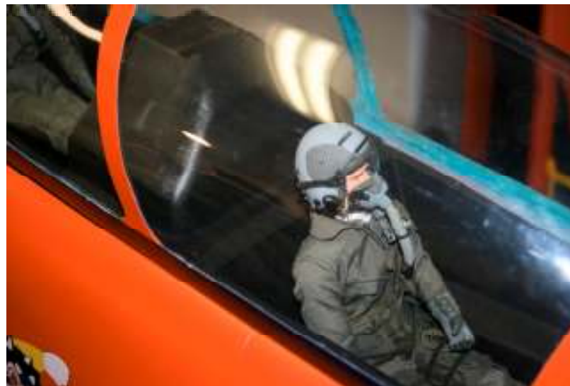
photo 33 – front tub glued in place on top of canopy rails
